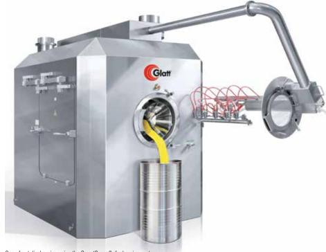
Open front discharging using the SmartScoop® discharging system
