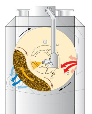
Principle of the Glatt coating process in the GC Master
