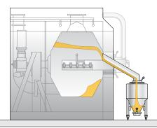
Closed front discharging into a container for an automatic process
