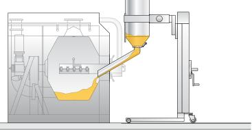
Front charging with an inlet pipe
