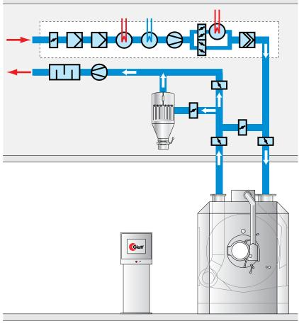
Glatt coater with the once-through principle with inlet and outlet air treatment
