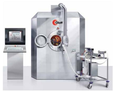
Glatt coater GC Master with horizontal drum, equipped for film coating
