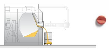
Open front discharging using the  ${\rm SmartScoop}^{\otimes}$  discharging system
